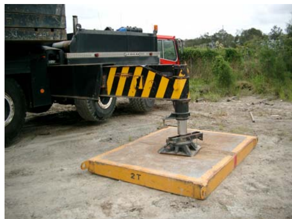
Figure 4 - Crane outrigger foot on bog mat
