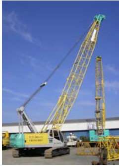
Figure 6 – Lattice boom crawler crane
