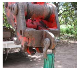
Figure 7 and Figure 8 - Lifting attachment with a closed eye on excavator
